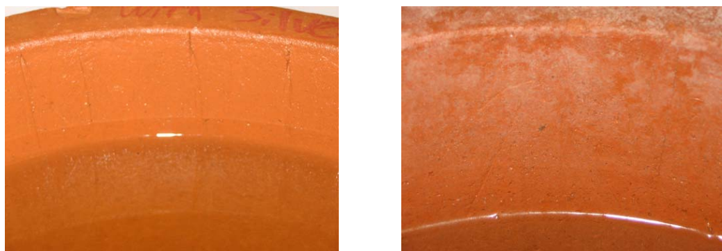
Figure 1.10 (a) No white 'rash' on filter with silver and (b) rash on filter without silver
