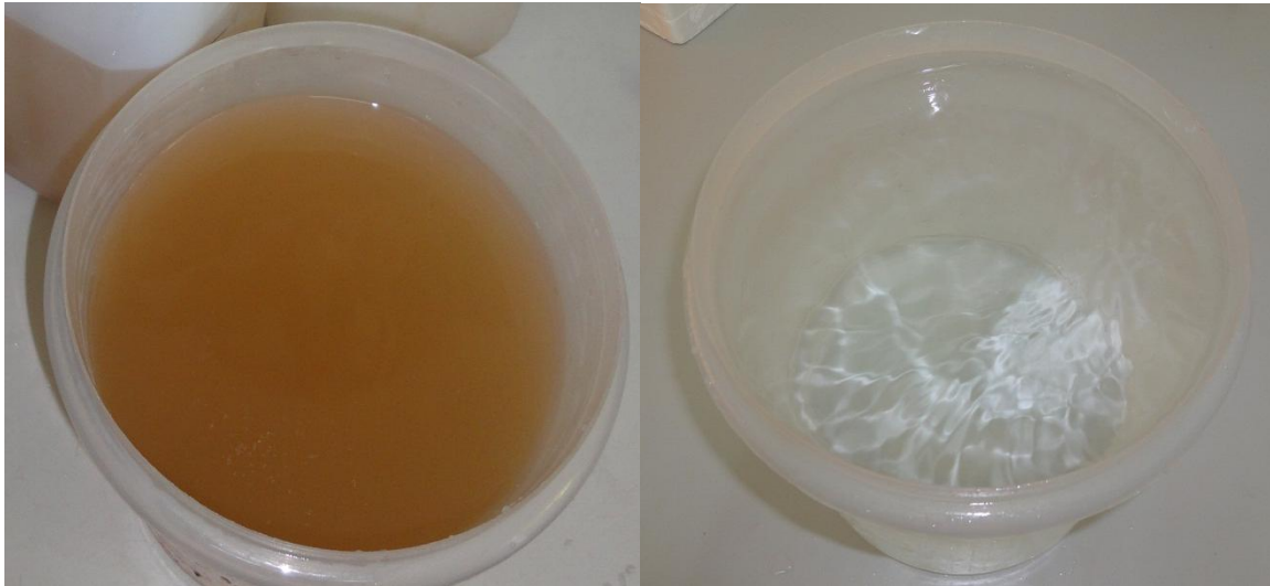
Image 1: Water sourced from a MSABI well - high in iron content - before and after filtration using a MSABI filter pot
