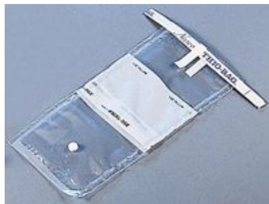
A WhirlPak™ sample collection bag (with a thiosulfate tablet to inactivate any chlorine present)
